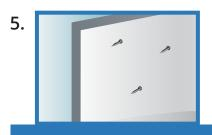
Fix the insulation over the pins
