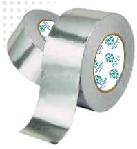
A nominal 30 micron (1.2 mil) high tensile strength aluminum foil backing, combined with a high performance solvent synthetic rubber-resin adhesive, protected by an easy-release silicone release paper.
