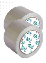
A laminated PET-Foil backing (Polyester: 12 Microns / Foil: 7 Microns), combined with a high performance solvent acrylic adhesive, protected by an easy-release silicone release paper.
